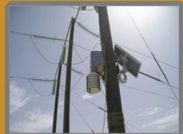
Pollution Monitor on 132kV Wood Pole
